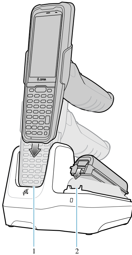
Figure 22 1-Slot Charge/Communication Cradle with Spare Battery Charger
