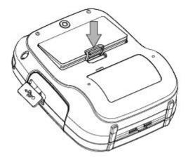
3. To remove the battery back, pull back the hook, and use the opposite procedure from the one you used to insert the battery pack.
